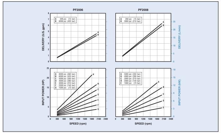
Typical performance curves are based on 100 SUS (20 cSt) mineral oil with pressurized inlet where required. Refer to the "Minimum Inlet Pressure" table on page 4.
