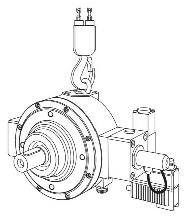
Fig. 17: Transporting Pump with Lifting Tackle
