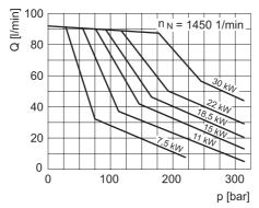
Fig. 14: Characteristic  $V = 63 \text{ cm}^3/U$
