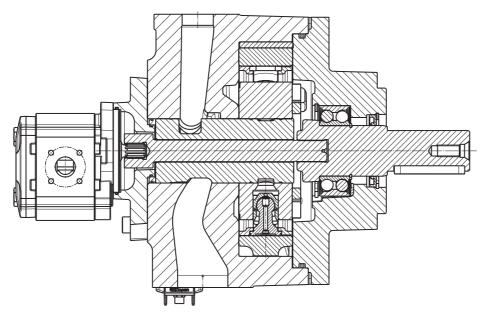
Fig. 20: Radial Piston Pump with Add-On Gear Pump SAE-A Adapter
