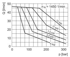
Fig. 13: Characteristic  $V = 32 \text{ cm}^3/U$
