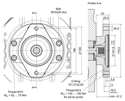
Fig. 23: Adapter flange SAE-A with 13-tooth Shaft
