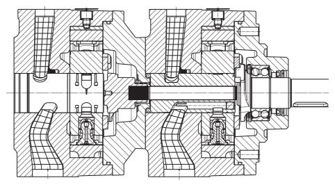
Fig. 19: Radial Piston Pump with Heavy Through Drive and Add-On Radial Piston Pump
