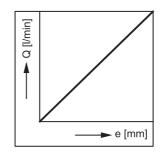
Mechanical Stroke Adjustment, B1
