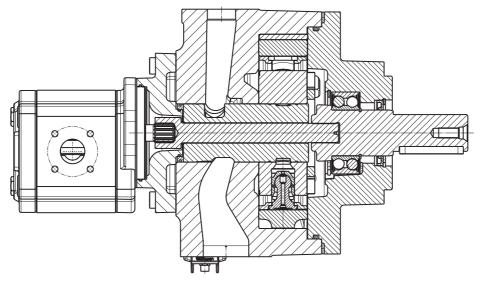
Fig. 21: Radial Piston Pump with Add-On Gear Pump SAE-B Adapter
