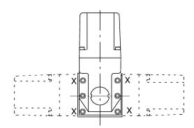
Amplifier and solenoid may be rotated 90° as shown by removing 4 screws shown X. Re-torque to 7-9 Nm (6-7 lbf ft)
