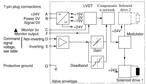
▲ Note: In valves with PH7 or PR7 type electrical connection, pin C is used for a valve enable signal.
