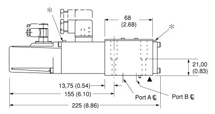
▲ Mounting surface seals supplied \*Note: Bleed screw locations Air bleed, Socket Head Cap Screw. Torque to 2,5-3,0 Nm (2.0-2.5 lbf ft)
