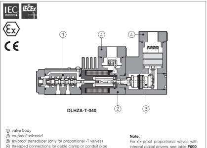
On/off and proportional valves equipped with explosion-proof solenoids available with following certifications and protection modes:
