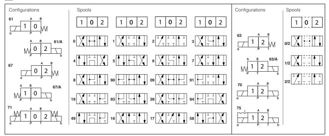
Note: spools 1, 1/2 and 3 are available as 1P, 1/2P and 3P to limit the valve internal leakage
