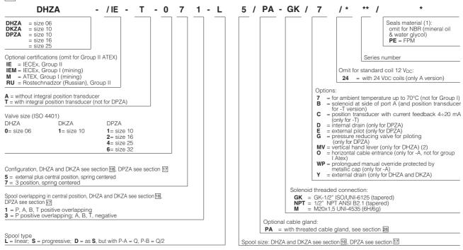
(1) Option /BT = low temperature -40°C also available on request only for valves -A without integral position transducer (not for group I Atex -mining-)
