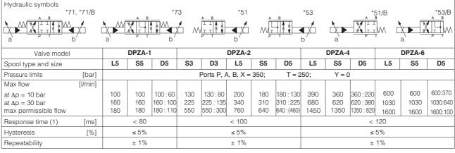
(1) Response times at step signal (0%→100%) are measured from 10% to 90% of step value and are strictly referred to the valve regulation.
