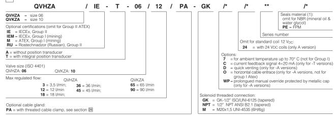
(1) Option /BT = low temperature -40°C also available on request only for valves -A without integral position transducer (not for group I Atex -mining-)
