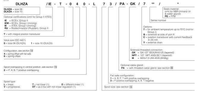
(1) Spool type D, DT and T are available only for valve with fail safe position DLHZA-\*-040 and DLKZA-\*-040
