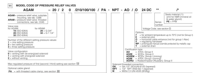
(1) Option  $\mbox{/BT} = \mbox{low temperature -} 40^{\circ}\mbox{C}$  also available on request (not for group I Atex -mining-)
