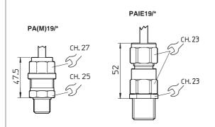
The cable glands PA and PAM, are available on request certified ATEX according to EN 60079-0 and EN 60079-1.
