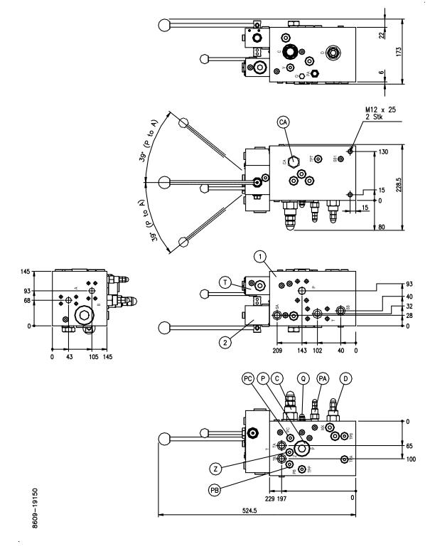
Figure 4 Dimensions 8MB-\*\*\*-2C-T-MA
