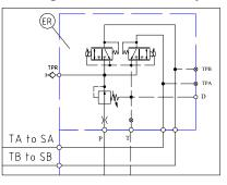
**Code L** Manual control safety lock for locking in 0 position only. This is a mechanical device for preventing operation of the directional valve unless the safety lock is manually released.
