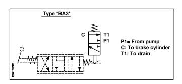
Code 37E Manually/Proportionally electrical remote operated. Proportional reducing valve item E is Hydranor 8FGB4131021-11/11. Pressure reducing valve not integrated in 8FGB4131021-11/11, but separate sandwich component.
