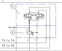
**Code 37ER** Manually/Proportionally electrical remote operated with integrated pressure reducing valve and external drain port D. T from ER to main block is plugged. Proportional reducing valve item ER is Hydranor 8FGBR4431021-11/11-D
