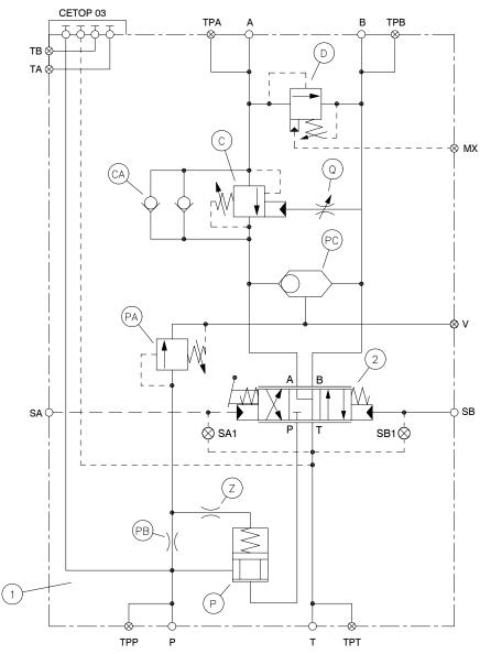
Figure 2 Hydraulic Schematic 8MB-200-37-2C-MA
