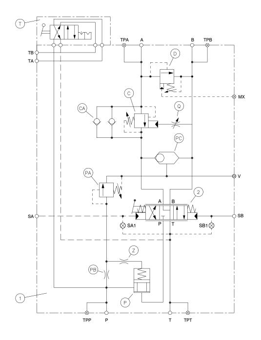
Figure 3 Hydraulic Schematic 8MB-\*\*\*-37-2C-MA-T
