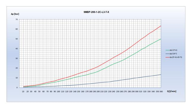
Figure 4 9MB-200-\*\*-2C-MA pressure drop
