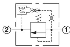
The -8 control option allows a pilot control valve to be incorporated directly into the end of the modulating element via the T-8A cavity. These pilot control cartridges are sold separately and include electro-proportional, solenoid, air pilot, and hydraulic pilot operation. See Pilot Control Cartridges on page 121.
