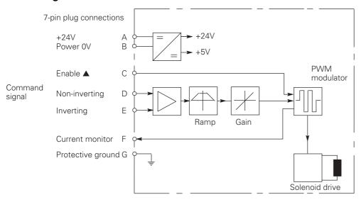
▲ In valves with PH7 or PR7 type electrical connection.
