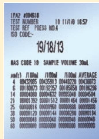
3 Online-dynamic Three Test & Result Average. ISO 4406 code.
