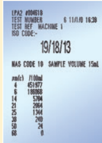
1 Online-normal Single test result. ISO 4406 code.
