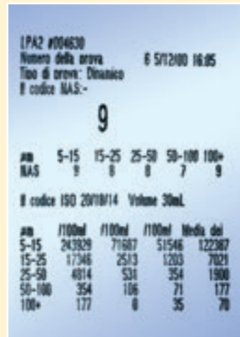
2 Online-dynamic Three test & result average. NAS 1638 code.
