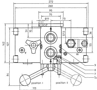
Pos. I: left filter-side in operation Pos. II: right filter-side in operation Connection V and VI to be used to bleed filter or to relieve pressure
