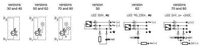
$p_1$  = measure connection supply  $p_2$  = measure connection output
