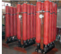
EXAMPLES OF BLADDER ACCUMULATOR STATIONS
