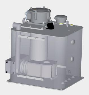
The Cyclone element comes in two different sizes. One dimensioned for returnflow up to 650 l/min  $(250 \times 130 \times 185 \text{ mm})$  and another for 350 l/min  $(250 \times 75 \times 185 \text{ mm})$ .
